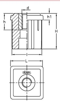
$\begin{array}{lll} d & = M10 \\ h & = 20 \\ H & = 33 \\ h1 & = 6 \\ Internal tube size = 27 \\ I & = 27.5 \\ L & = 30 \\ Outer tube size & = 30 \\ \end{array}$
